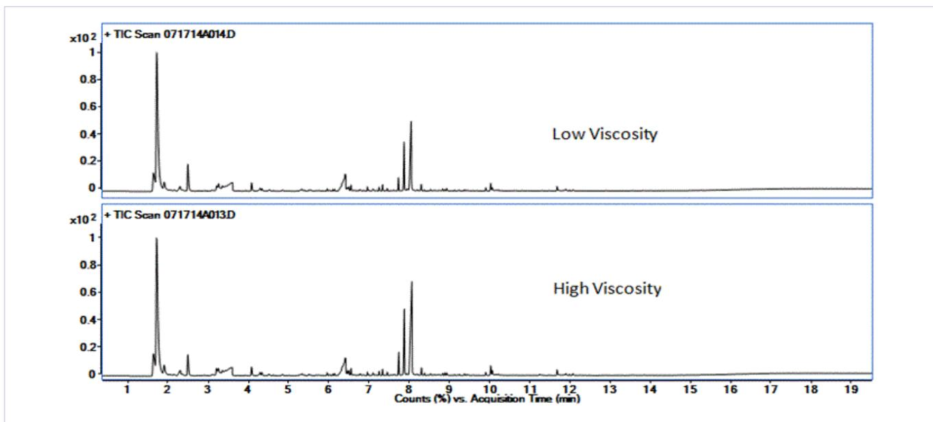
Figure 2: Pyrolyzate Profile Comparison of Low and High Viscosity 85/15 Lactide/ Caprolactone Copolymer Resin
