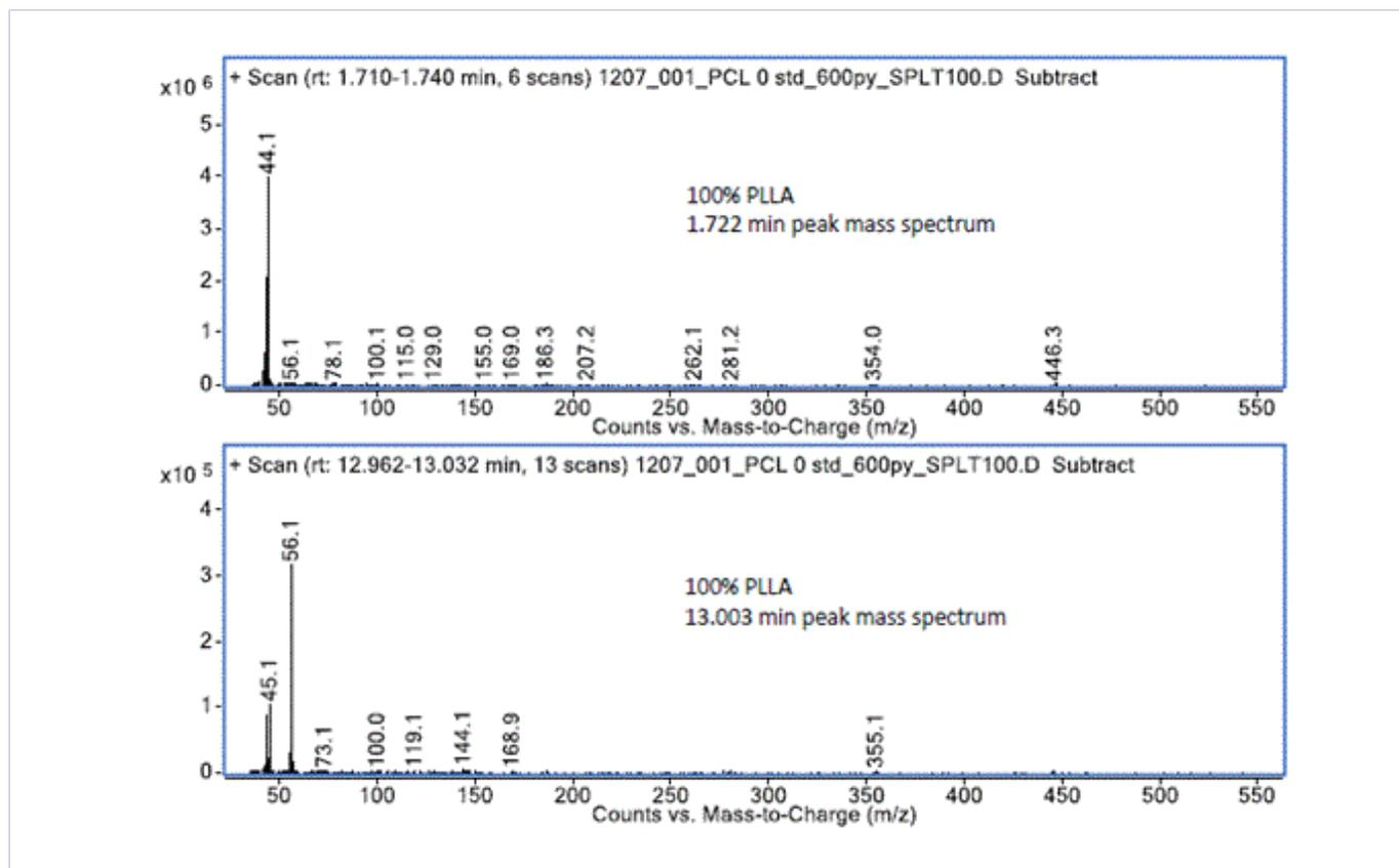
**Figure 6:** Spectra of Peaks at Retention Times of 1.7 and 13.0 Minutes Selected for PLLA Quantification
