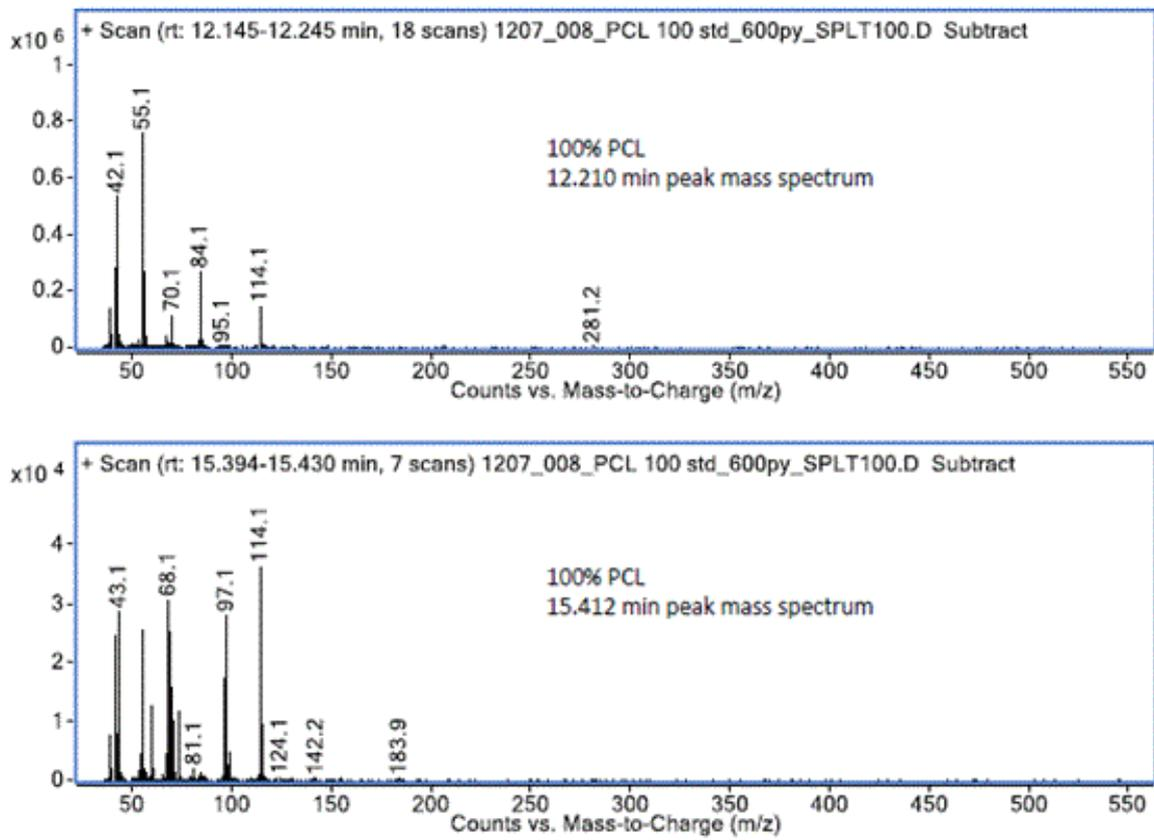
Figure 4: Mass Spectra of 12.210 and 15.412 Minute Retention Time Peaks Selected For PCL Quantification
