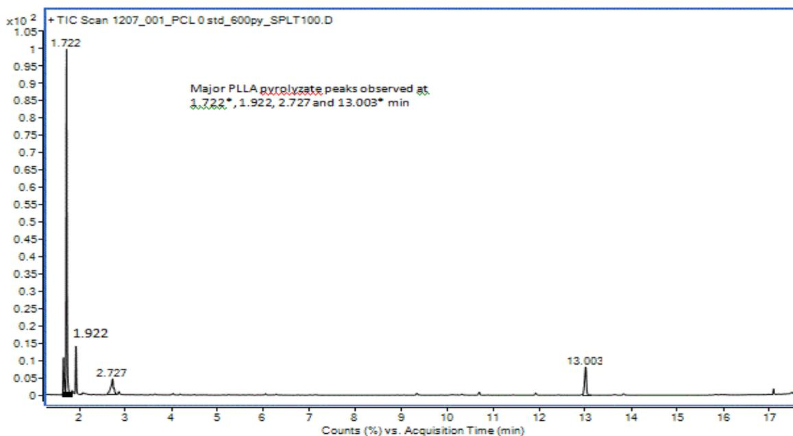
Figure 5: Total Ion Current GC/MS Pyrogram of 100% Poly (Lactide) Resin \*Peaks Selected for Quantification of Lactide Amount
