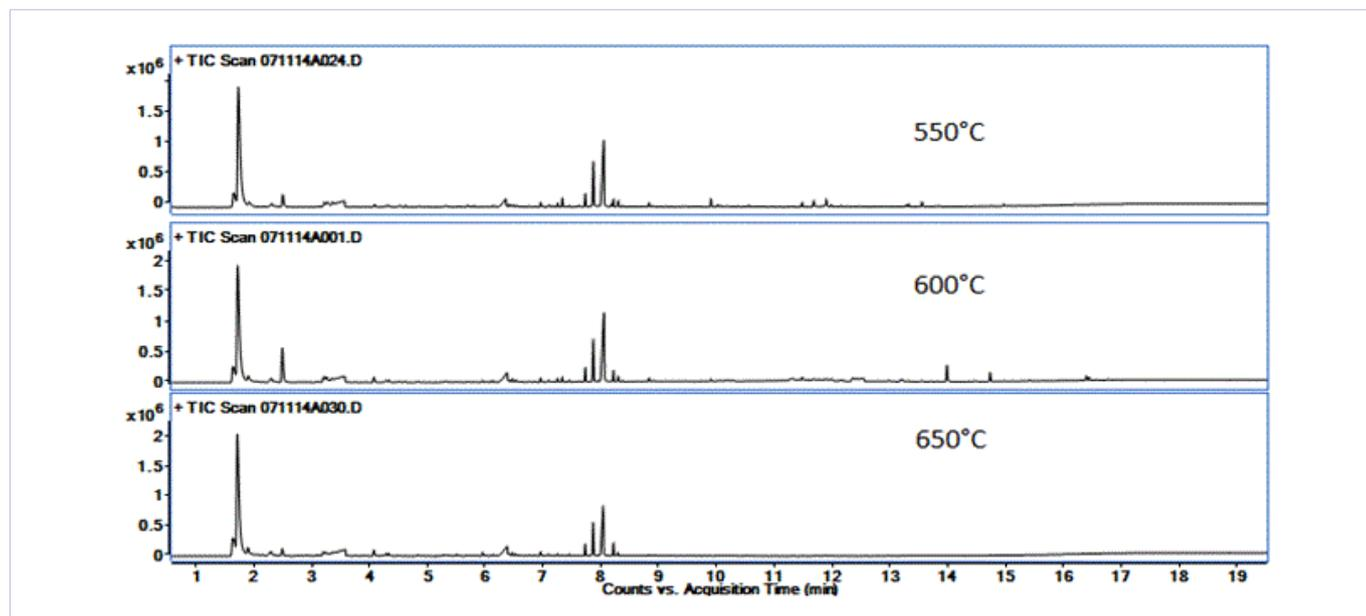
Figure 1: Effect of Temperature on the Pyrolyzate Profile
