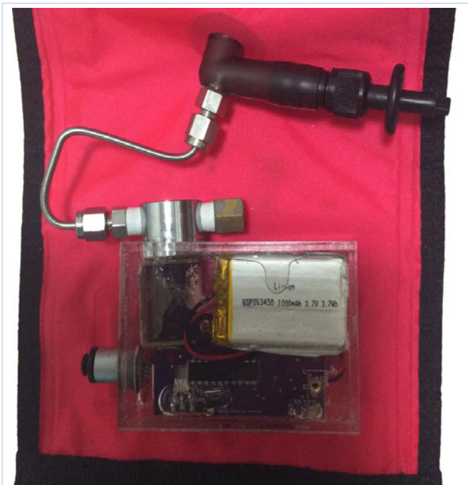
Figure 5: Assembled ART unit ready for attachment of CO 2 cartridge and deployment.
