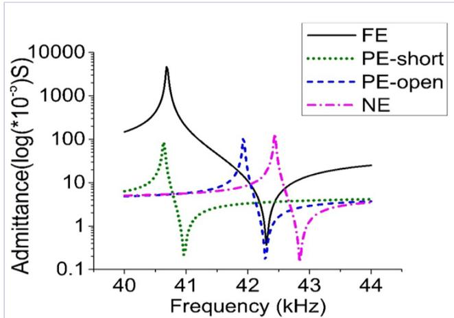
Figure 3: Experimental Results - Admittance spectrum of the full and partial electrode samples.
