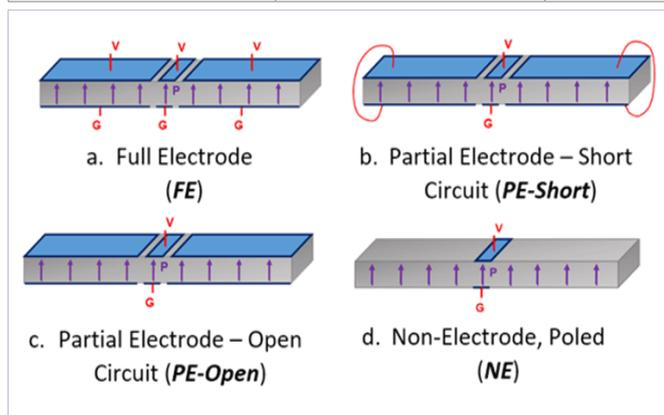
**Figure 2:** Schematic view of (a) full-electrode (FE), (b) partial electrode - short-circuit, (c) partial electrode - open circuit, and (d) non-electrode (NE) samples.
