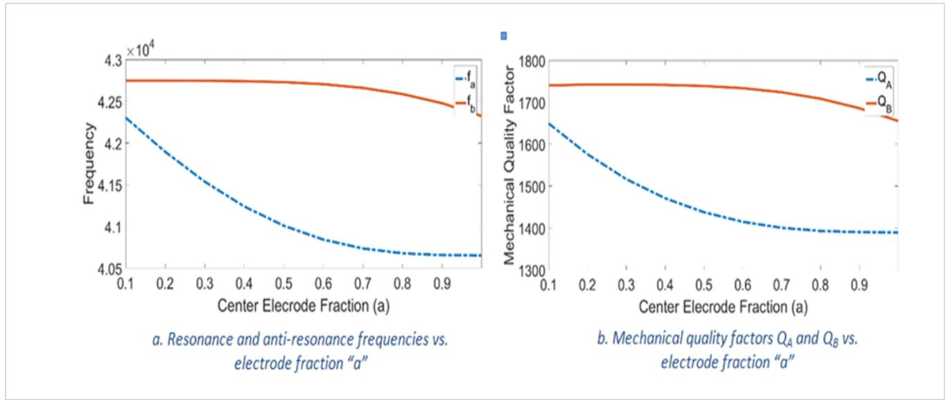
**Figure 8:** Effect of the center electrode area on the resonance and anti-resonance frequencies and their corresponding mechanical quality factors.
