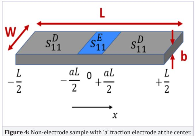
Figure 4: Non-electrode sample with 'a' fraction electrode at the center.
