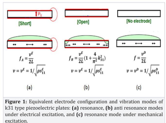
**Figure 1:** Equivalent electrode configuration and vibration modes of  $k_{31}$  type piezoelectric plates: (a) resonance, (b) anti resonance modes under electrical excitation, and (c) resonance mode under mechanical excitation.
