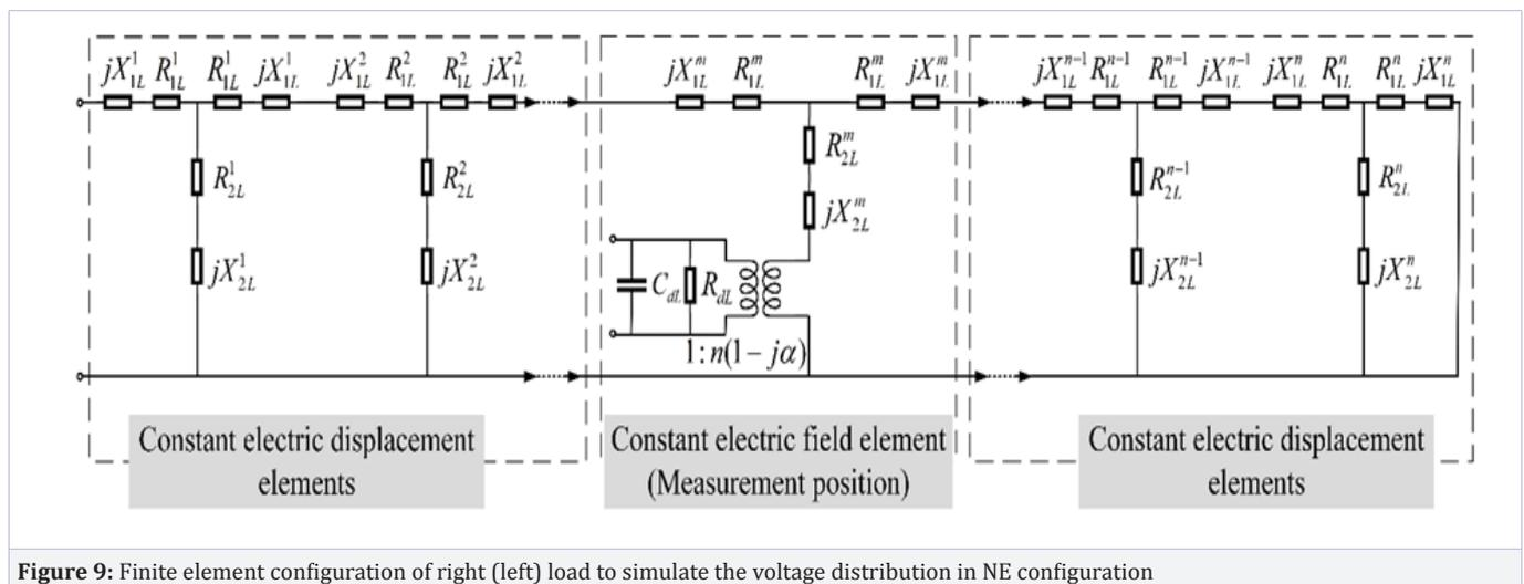
**Figure 9:** Finite element configuration of right (left) load to simulate the voltage distribution in NE configuration
