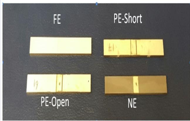
**Figure 5:** (a) full-electrode (FE), (b) partial electrode - short-circuit, (c) partial electrode - open circuit, and (d) non-electrode (NE) samples ( $a = 0.1$ ).
