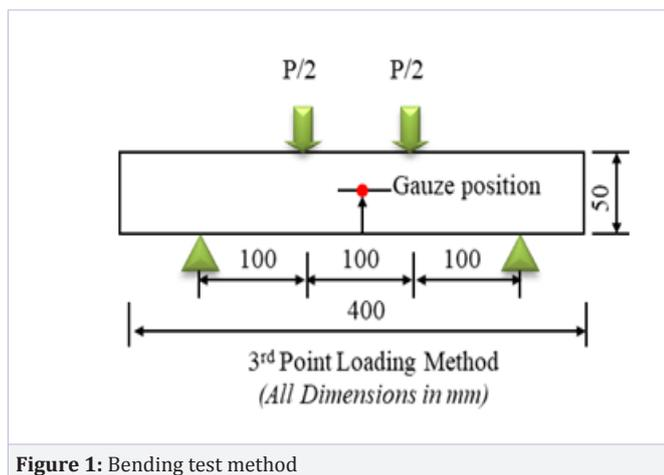
Figure 1: Bending test method
