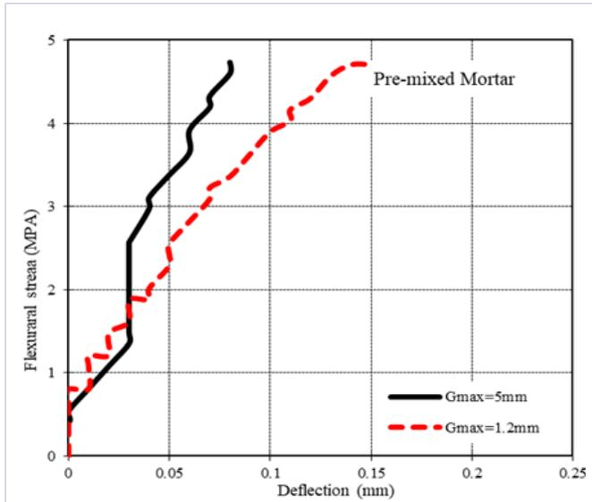
Figure 4: Close-up flexural stress- deflection relationship of pre-mixed mortar method up to 4.5 MPa
