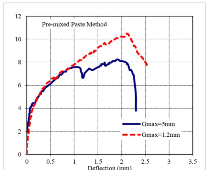
Figure 3: Flexural stress- deflection relationship of pre-mixed mortar mixing method
