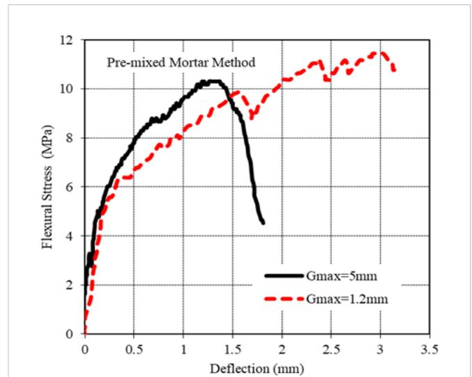
Figure 2: Flexural stress- deflection relationship of pre-mixed mortar mixing method
