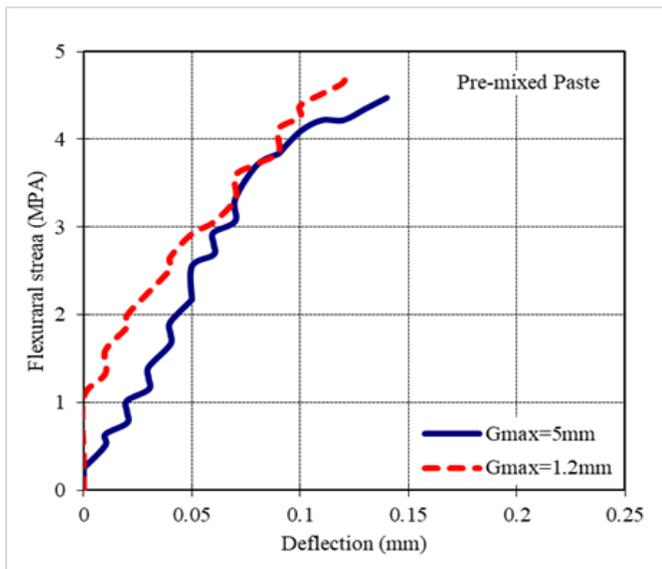
Figure 5: Close-up flexural stress- deflection relationship of pre-mixed paste mixing method up to 4.5 MPa
