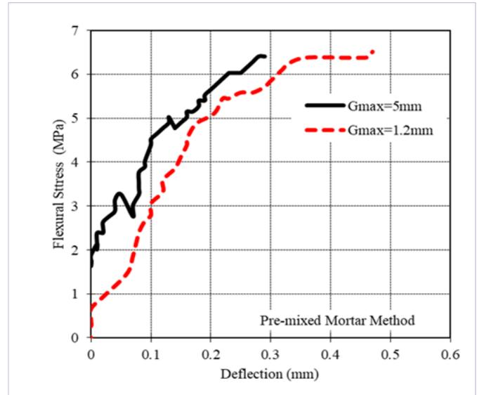
Figure 6: Close-up flexural stress- deflection relationship of pre-mixed mortar method up to 6.4 MPa
