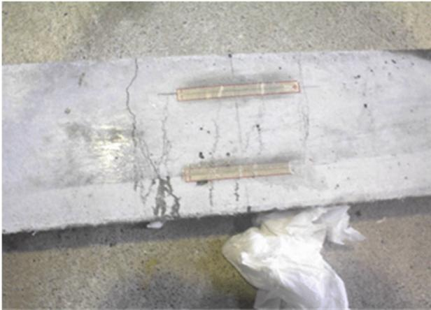
**Figure 8:** Condition of multi-cracks on bottom surface of specimen after completion of bending test
