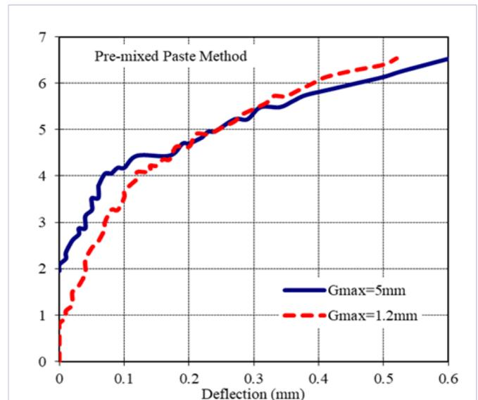
Figure 7: Close-up flexural stress- deflection relationship of pre-mixed paste mixing method up to 6.4 MPa
