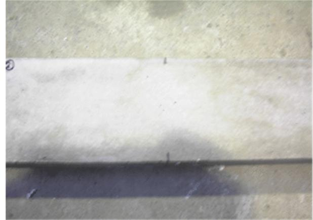
**Figure 9:** Condition of the bottom surface after flexural stress reached to 6.4 Mpa in bending test
