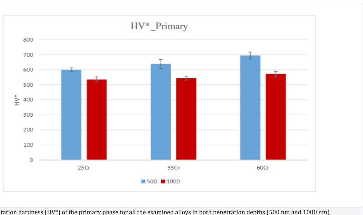
**Figure 4:** Indentation hardness (HV\*) of the primary phase for all the examined alloys in both penetration depths (500 nm and 1000 nm)
