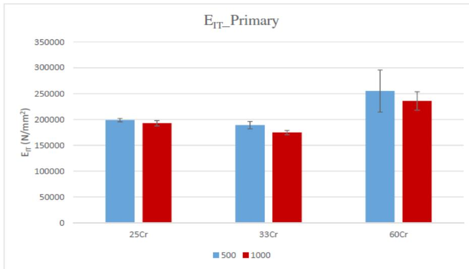
Figure 2: Indentation modulus ( $E_{IT}$ ) of the primary phase for all the examined alloys in both penetration depths (500 nm and 1000 nm)
