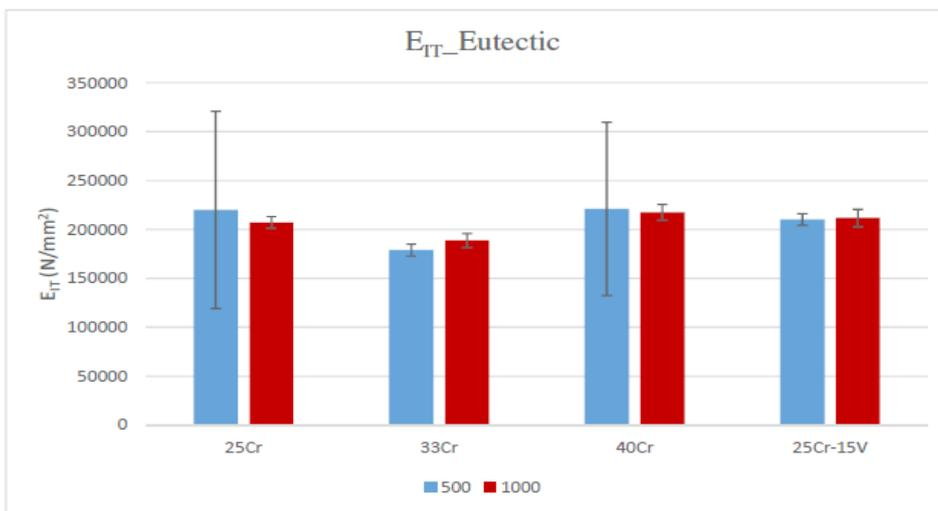
Figure 3: Indentation modulus ( $E_{IT}$ ) of the eutectic phase for all the examined alloys in both penetration depths (500 nm and 1000 nm)
