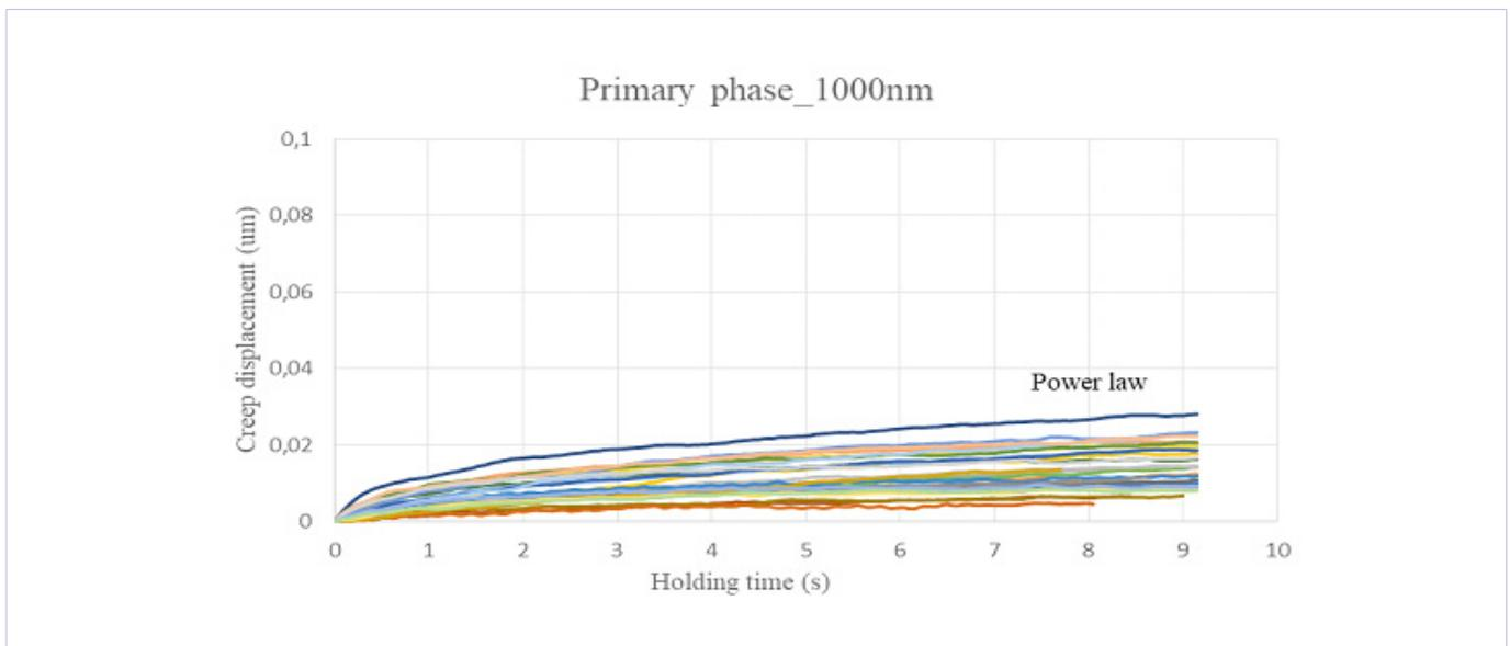
**Figure 14:** The indentation displacement as a function of time during the holding (creep) stage of the indentation tests for the primary phase at 1000 nm penetration depth
