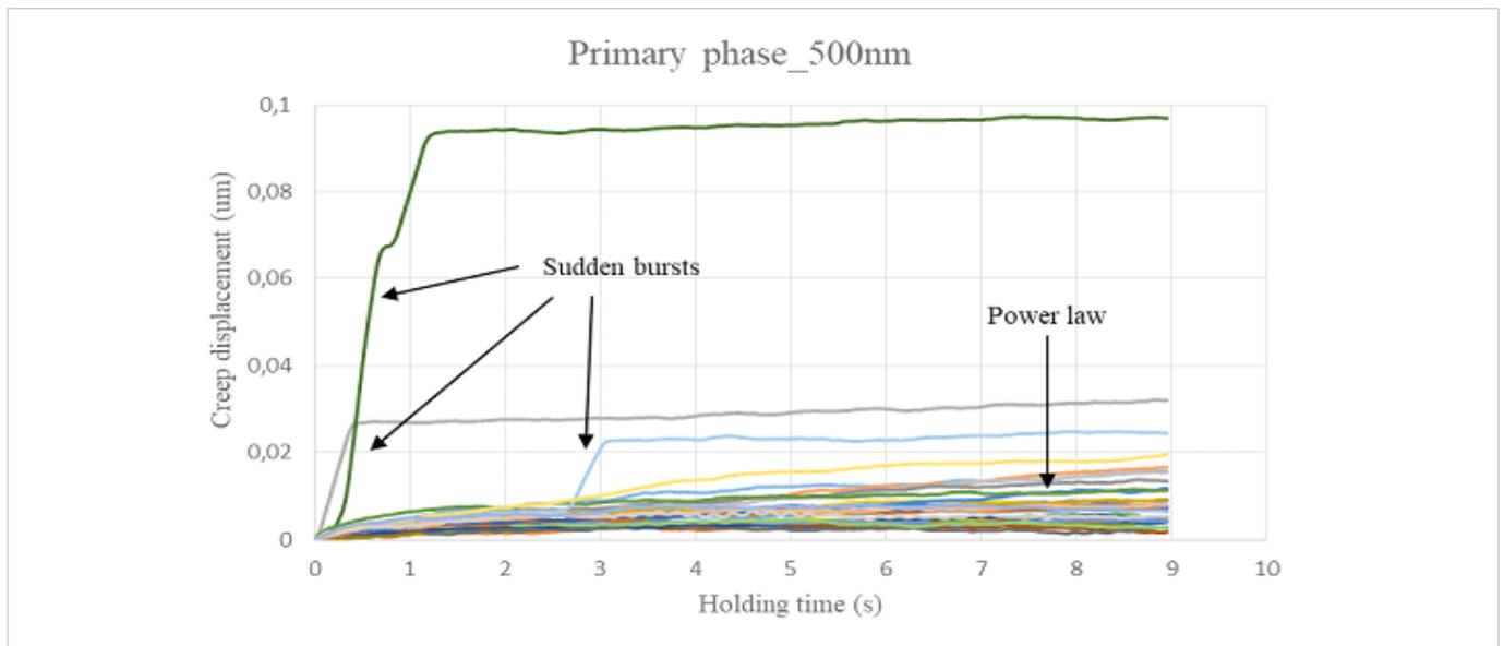
**Figure 12:** The indentation displacement as a function of time during the holding (creep) stage of the indentation tests for the primary phase at 500 nm penetration depth
