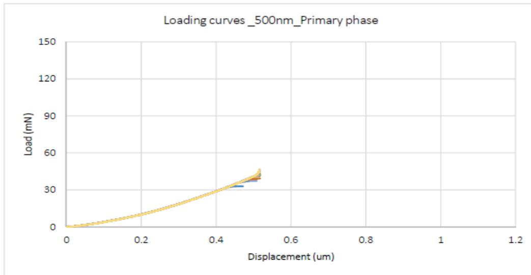
**Figure 8:** Loading curves of the primary phase at 500 nm penetration depth
