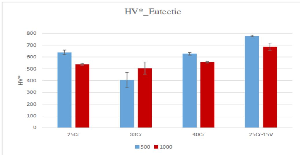
Figure 5: Indentation hardness (HV\*) of the eutectic phase for all the examined alloys in both penetration depths (500 nm and 1000 nm)
