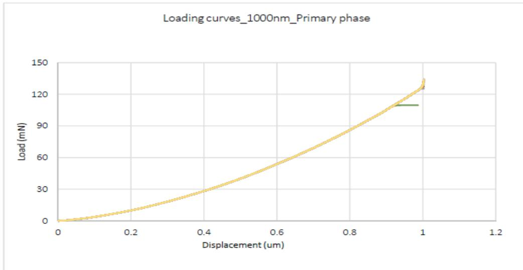
**Figure 10:** Loading curves of the primary phase at 1000 nm penetration depth
