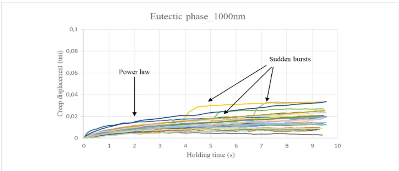
**Figure 15:** The indentation displacement as a function of time during the holding (creep) stage of the indentation tests for the eutectic phase at 1000 nm penetration depth
