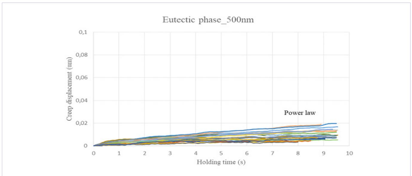
**Figure 13:** The indentation displacement as a function of time during the holding (creep) stage of the indentation tests for the eutectic phase at 500 nm penetration depth
