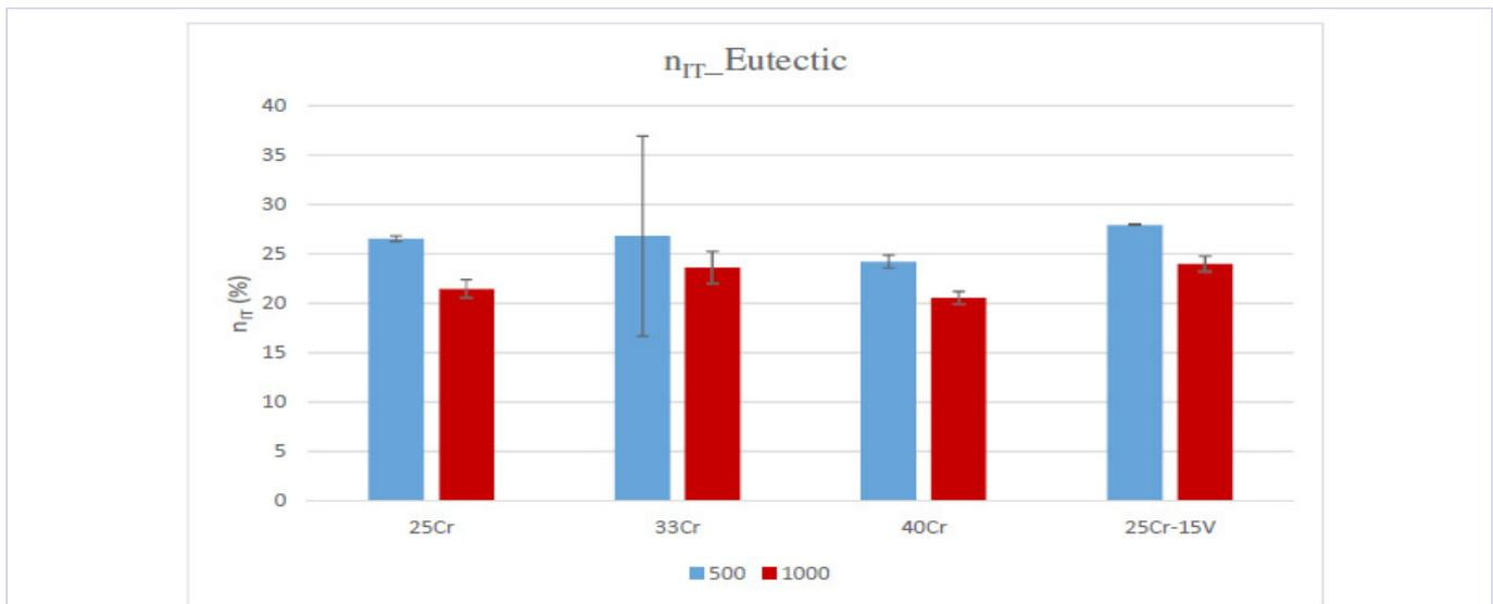
**Figure 7:** The percentage of the absorbed elastic energy compared to the total energy absorbed during the test ( $n_{TT}$ ), of the eutectic phase for all the examined alloys in both penetration depths (500 nm and 1000 nm)
