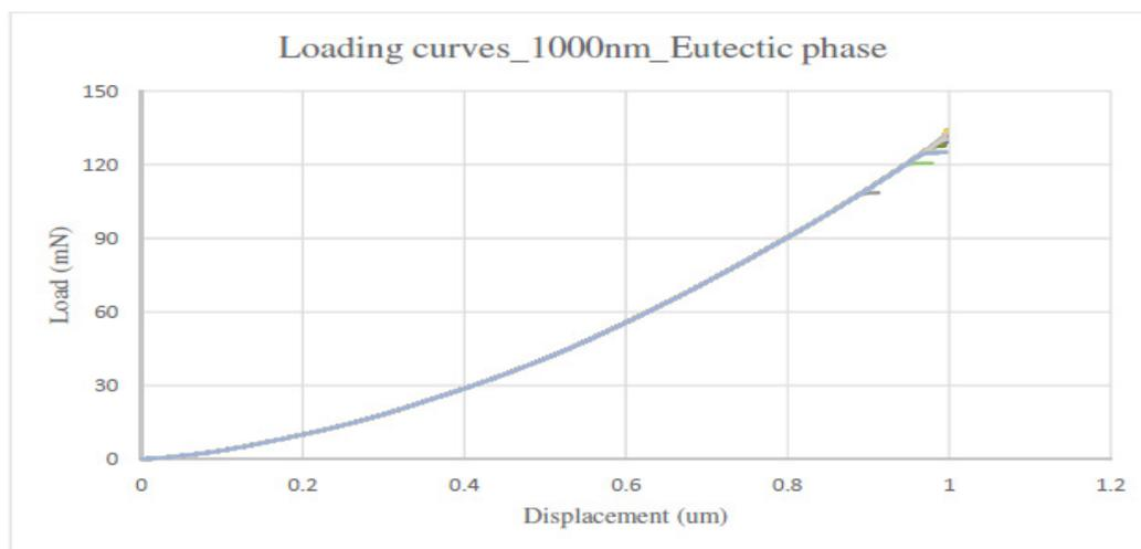
**Figure 11:** Loading curves of the eutectic phase at 1000 nm penetration depth
