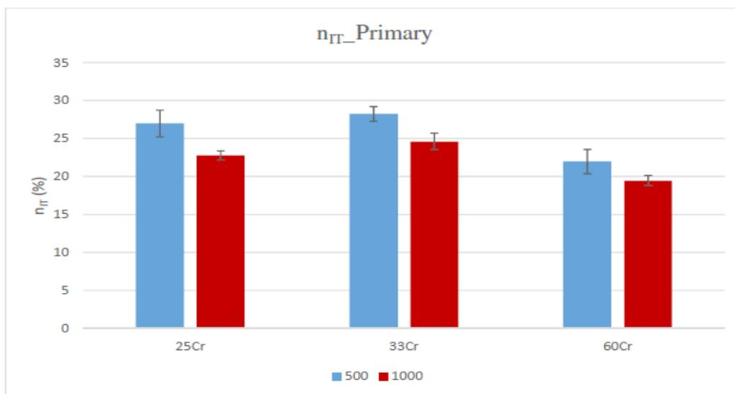
Figure 6: The percentage of the absorbed elastic energy compared to the total energy absorbed during the test ( $n_{IT}$ ), of the primary phase for all the examined alloys in both penetration depths (500 nm and 1000 nm)
