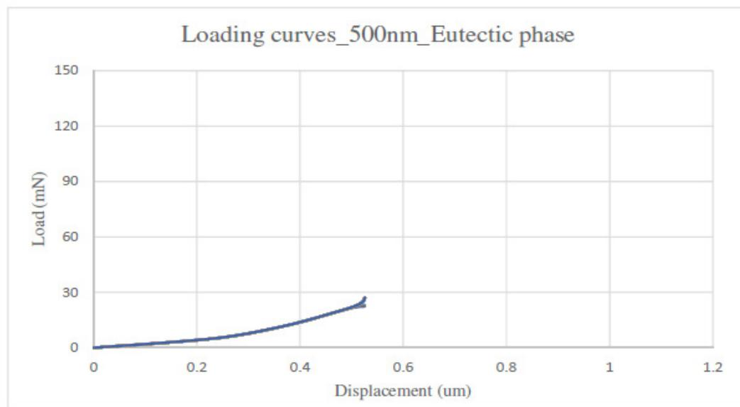
**Figure 9:** Loading curves of the eutectic phase at 500 nm penetration depth
