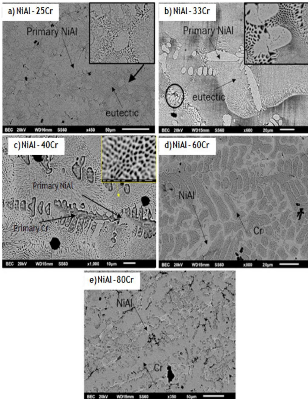
**Figure 1:** The panoramic view of the microstructure of the produced alloys: (a) NiAl-25Cr, (b) NiAl-33Cr, (c) NiAl-45Cr, (d) NiAl-60Cr and (e) NiAl-80Cr. Reconstruction after the work of Mathiou et al. [19]
