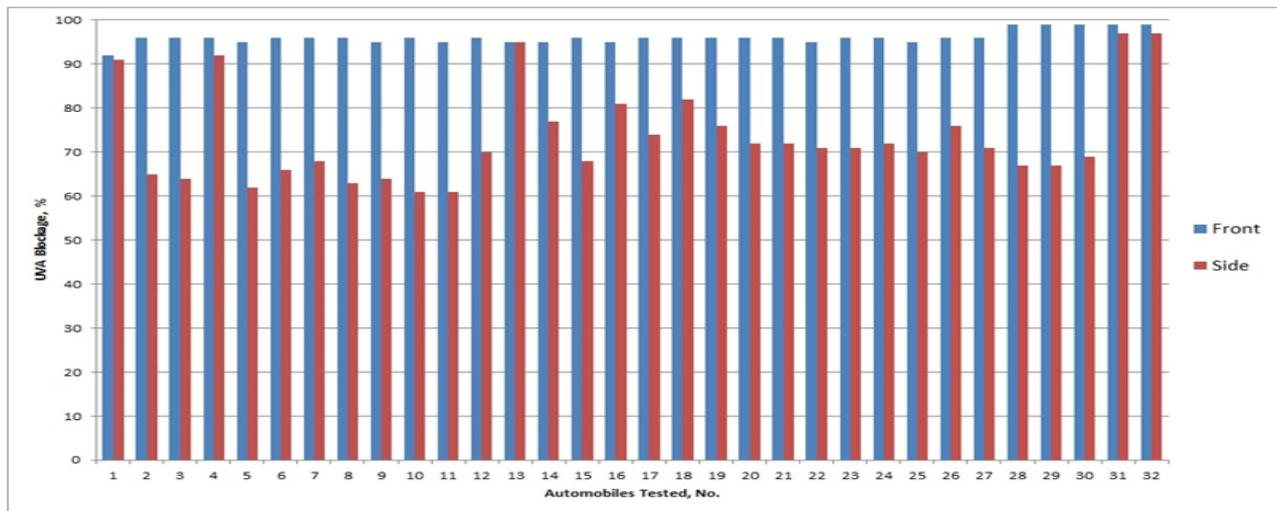
**Figure 4:** The distribution of front windshield UVA blockage was consistently highly compared to the more variable distribution of side window UVA blockage for same vehicles.
