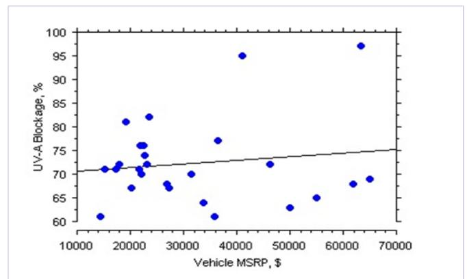
Figure 2: For 26 cars with MSRP under \$70,000 there was also no correlation of vehicle cost and side window UVA protection ( $r^2 = .02$ ,  $P = .50$ ).
