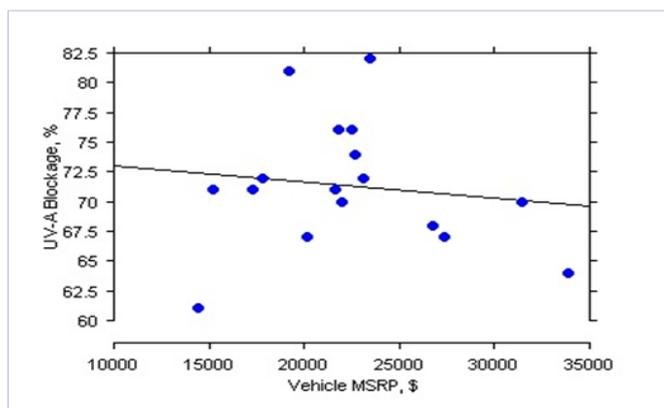
Figure 3: For 17 cars with MSRP under \$35,000 there was also no correlation of vehicle cost and side window UVA protection ( $r^2 = .02$ ,  $P = .62$ ).
