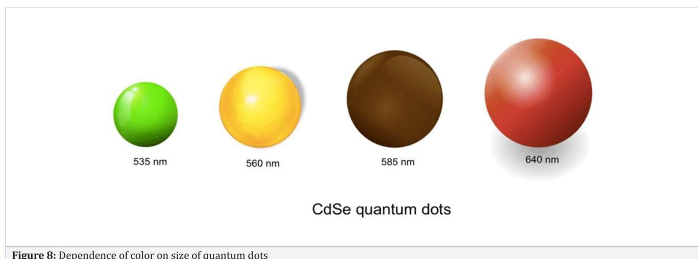
**Figure 8:** Dependence of color on size of quantum dots
