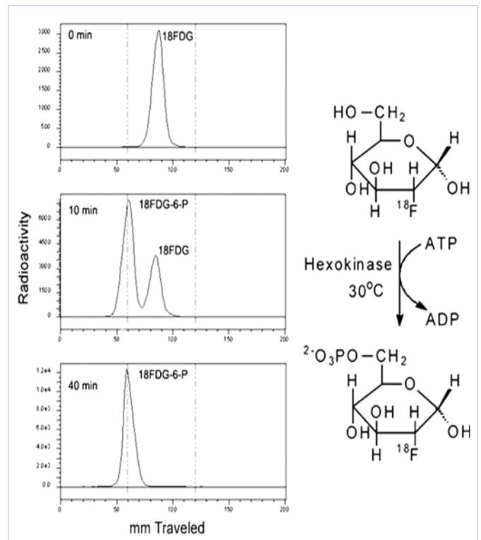
**Figure 2:** This figure shows the time course for *in vitro* enzymatic conversion of  $^{18}\text{F}$ FDG to  $^{18}\text{F}$ FDG-6-P. Radio thin layer chromatography was used to separate the two substrates. The same TLC method was used to analyze leaf tissue extract for extent of  $^{18}\text{F}$ FDG phosphorylation.
