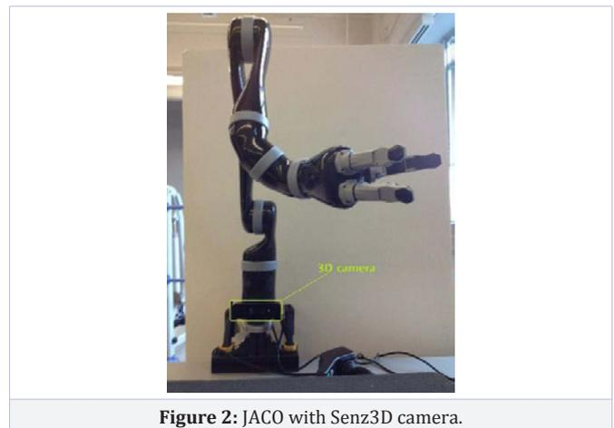
Figure 2: JACO with Senz3D camera.
