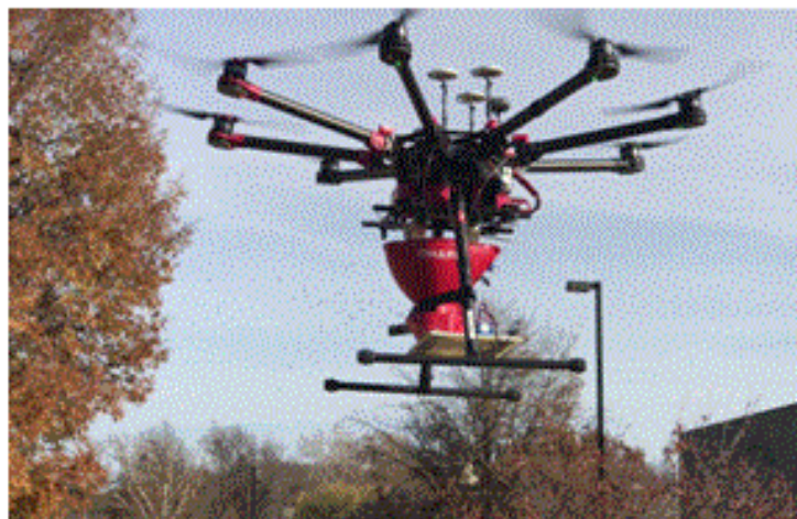
Figure 5: The prototype attached to the UAV distributing pupal parasitoid
