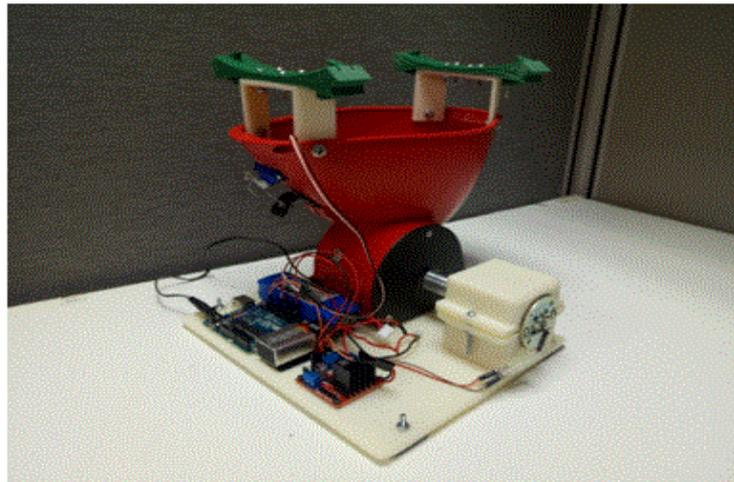
**Figure 2:** The prototype pupal parasitoid distribution device
