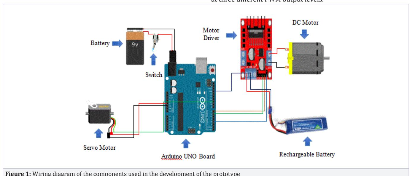
**Figure 1:** Wiring diagram of the components used in the development of the prototype
