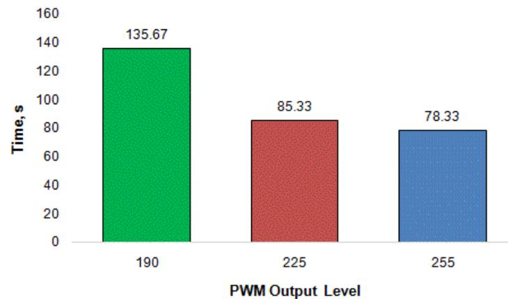
Figure 4: The average time it takes for the device to distribute the pupal parasitoids at different PWM output levels
