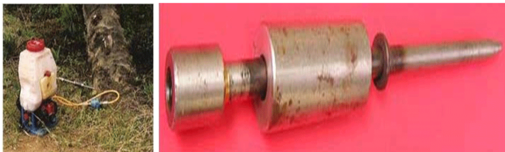
Plate 16: Control of Ganoderma in existing stand using fungicide hexaconazole trunk injection with hand knock injector which attached to the Motorized Knapsack Sprayer
