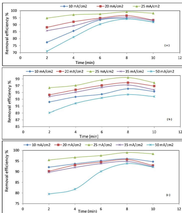
**Figure 1:** Effect of current density on the efficiency of styrene acrylic adsorption using iron (a), stainless steel (b) and aluminum (c) electrodes respectively
