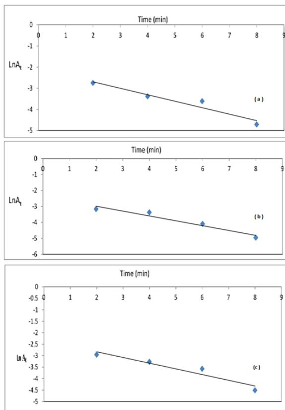
Figure 7: Relation between  $\ln A_t$  against the time for styrene acrylic adsorption using iron (a), stainless steel (b) and aluminum (c) electrodes respectively
