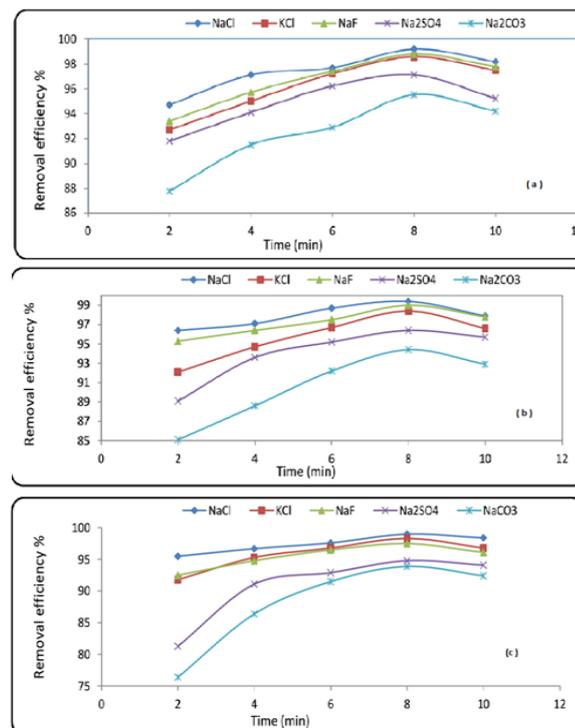
Figure 3: Effect type of electrolyte concentration on the efficiency of styrene acrylic adsorption using iron (a), stainless steel (b) and aluminum (c) electrodes respectively
