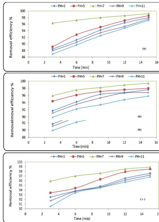
Figure 2: Effect of pH on the efficiency of styrene acrylic adsorption using iron (a), stainless steel (b) and aluminum (c) electrodes respectively
