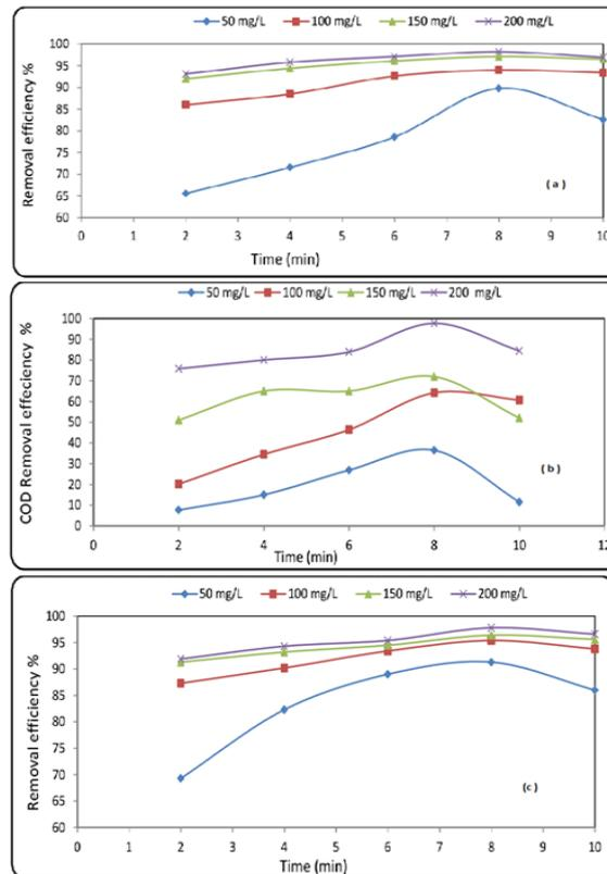
**Figure 5:** Effect of initial concentration on the efficiency of styrene acrylic adsorption using iron (a), stainless steel (b) and aluminum (c) electrodes respectively
