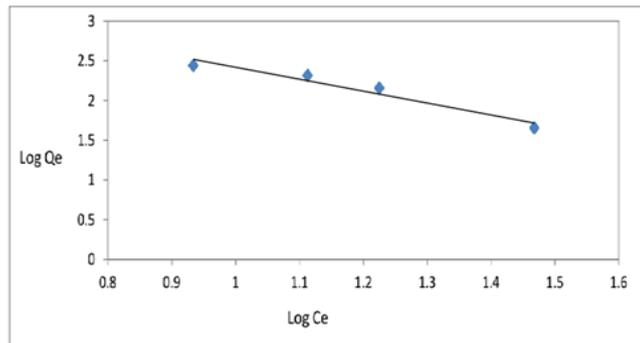
Figure 8: Freundlich plot (log qe vs. log Ce). for styrene acrylic adsorption using S.S electrodes
