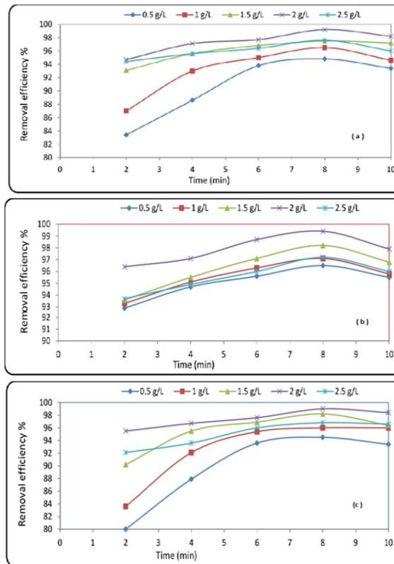
**Figure 4:** Effect of electrolyte concentration on the efficiency of styrene acrylic adsorption using iron (a), stainless steel (b) and aluminum (c) electrodes respectively
