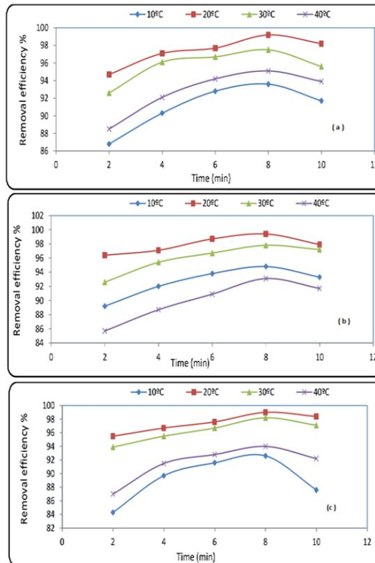
Figure 6: Effect of temperature on the efficiency of styrene acrylic adsorption using iron (a), stainless steel (b) and aluminum (c) electrodes respectively
